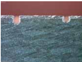
Plugged & Planerized, hole 0.2 mm
